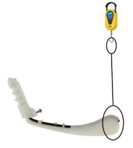
firmer has a tension screw add tension or replace if out of specs.
