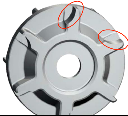
Worn drive pulley teeth – Should be replaced
