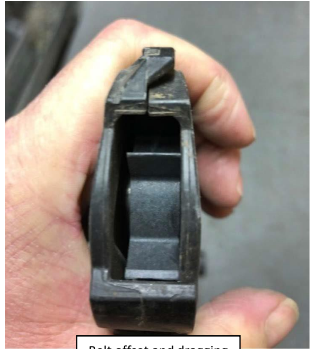
Belt offset and dragging causing high friction
