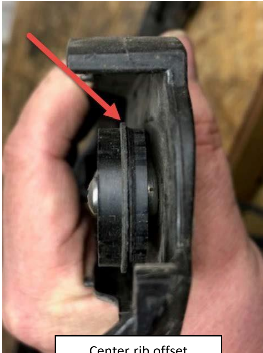
Center rib offset pushing belt to one side
