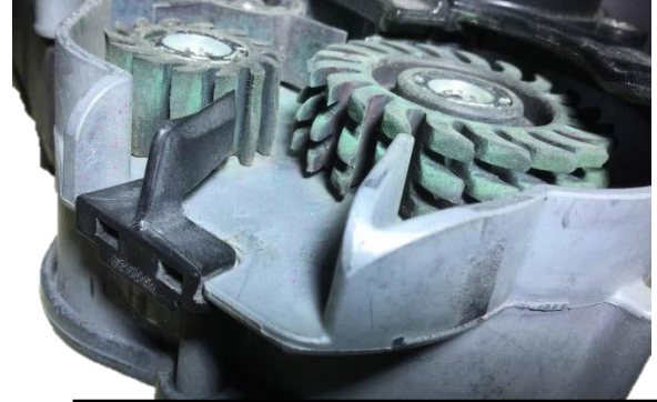
Bumps worn off on feeder wheels on side closest to seed disk— Should be replaced if wear is present effecting SRI.
