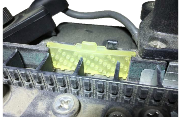
New insert installed in housing
