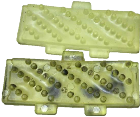
New housing insert (top) vs. worn housing insert (bottom) – Replace when bumps are worn down/broken off
