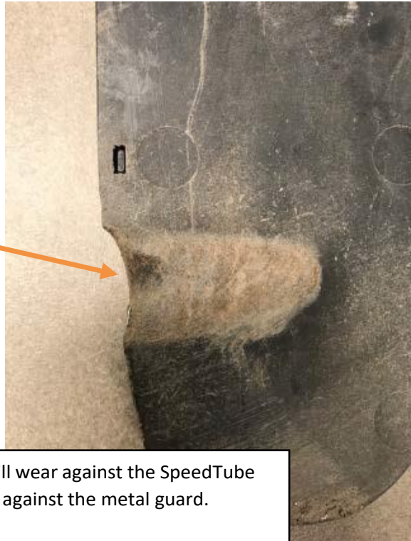
The SpeedTube housing will stop wearing once it meets the cast guard.
