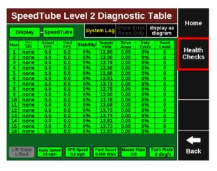
Speed Source-Will display current speed source "GPS", "Radar", or "none".
