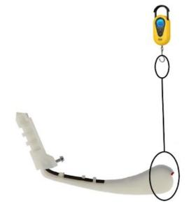
Quick Attach firmers are non-adjustable regarding tension Use flatness or droop (lack of tension) for replacement test
