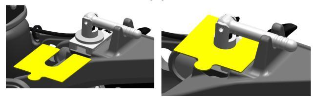
If the provided shim gauge is not available, any object with the appropriate thickness (0.050–0.060") can be used in the same fashion to check the clearance between the washers and the depth handle shoulder.
