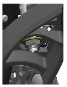
Note: The following step is CRITICAL to insure proper final installation and thus operation of the FurrowForce load sensor. Incorrect washer to sensor clearance will result in incorrect readings from the sensor.
