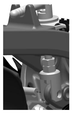
Rotate the tail frame up and unthread the depth yoke assembly (1) from the depth handle assembly. Use a socket to remove the locknut (2).
