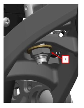
Lift the depth adjustment handle and remove it from the casting. Remove the old belleville washers.
