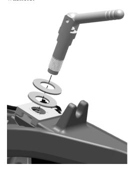
Install the new belleville washers on top of the FurrowForce load sensor.
