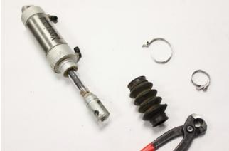
**Step 2:** Slide the new bellow onto the fully extended cylinder rod.
