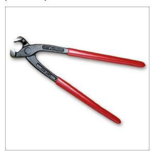
**Step 1:**Remove the clamps securing your damaged bellow. This is accomplished by anchoring the crimping tool around the crimped portion of the clamp, and then lift up the clasp portions of the clamp.
