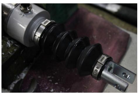
**Step 3:** Crimp the clamps on both sides of the bellow.
